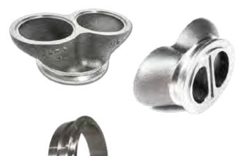
**Divided Vband Inlet Adapter:** The Garrett divided V-band adapter is for enthusiasts that are fabricating divided exhaust manifolds. This adapter mates perfectly with GT/GTX 30 and 35 divided Vband turbine housings and has two 2" recessed orifices that feed into the flange.
